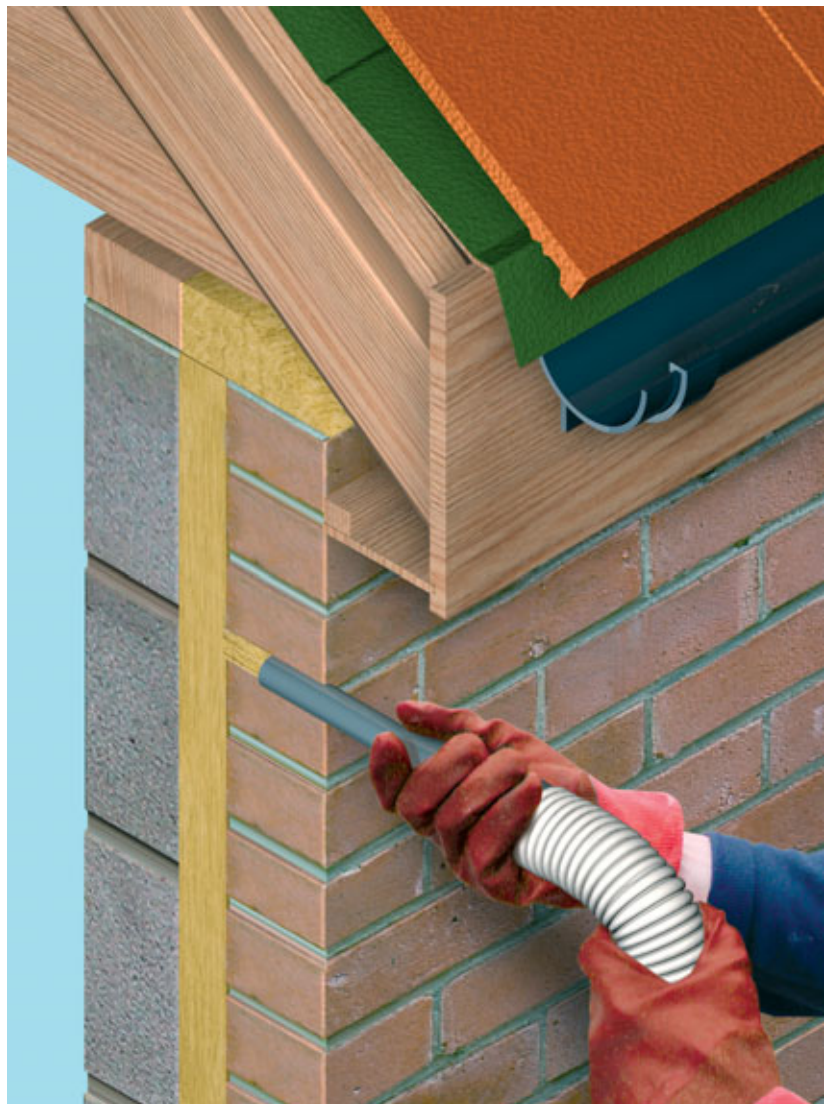
Installation of Rockwool EnergySaver into traditional brick/block cavity wall
